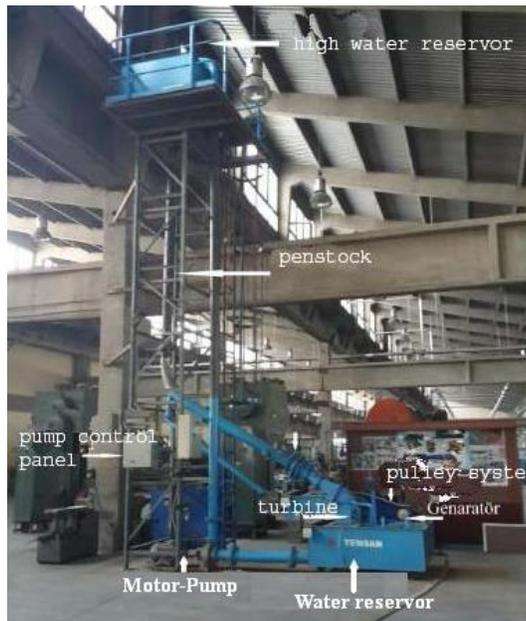
**Figure 2.** hydro-mechanical section general appearance.
