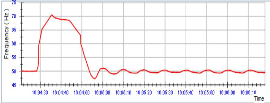
**Figure 8.** Frequency variation for load shedding, % 100
